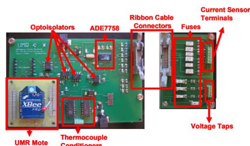
Fig. 1. UMR Power Monitoring Board
