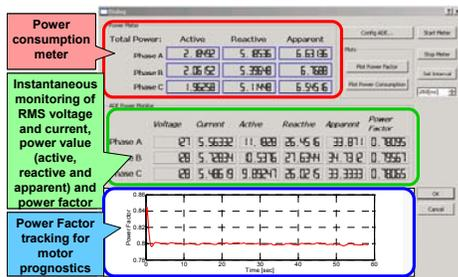
**Fig. 2. Power Monitoring GUI**
