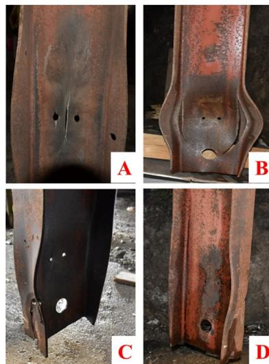
**Figure 5.** (A) damage to the column from the traditional dynamite charge (B) Damage to the column from the water-cased charge (C): Damage to the column from the half water-cased charge (D): Damage to the column from the quarter water-cased charge.
