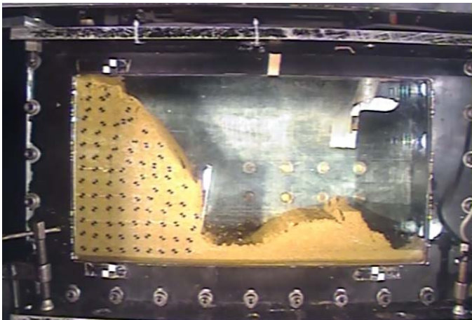
(c) Failure at 36 g
