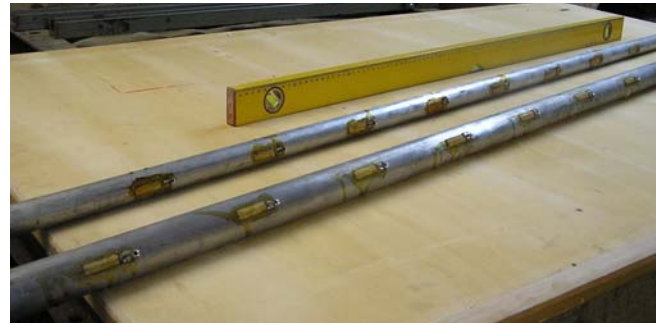
Fig.2 Appearance of piles equipped with strain gauges
