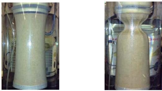
Fig. 2. Failure modes of loose and dense sand.
