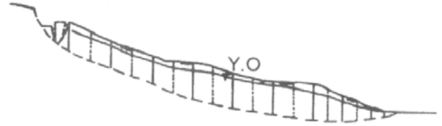
Fig. 4. The water table location (YO) and location of the slip surface at the slope (Georgopoulos and Vardoulakis, 2001)
