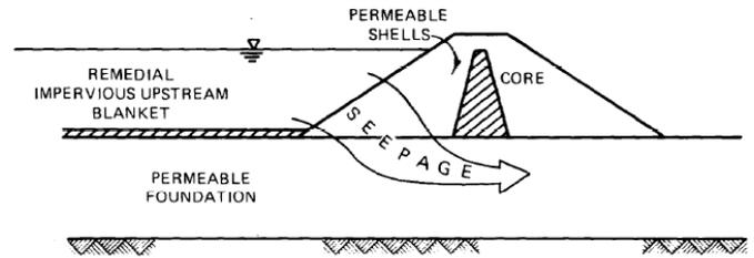
Fig. 2. Under-seepage Through Permeable Foundation (From USACE, 1986)
