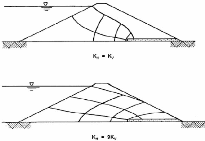
Fig. 5. Effect of  $k_h:k_v$  Ratio on Seepage Line
