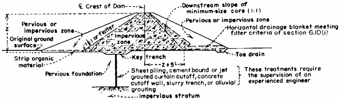
(B) INTERMEDIATE DEPTH OF PERVIOUS FOUNDATION
