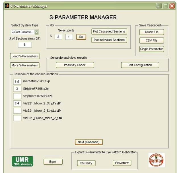
Figure 10. S-Parameter Manager window for cascading the S-parameters.
