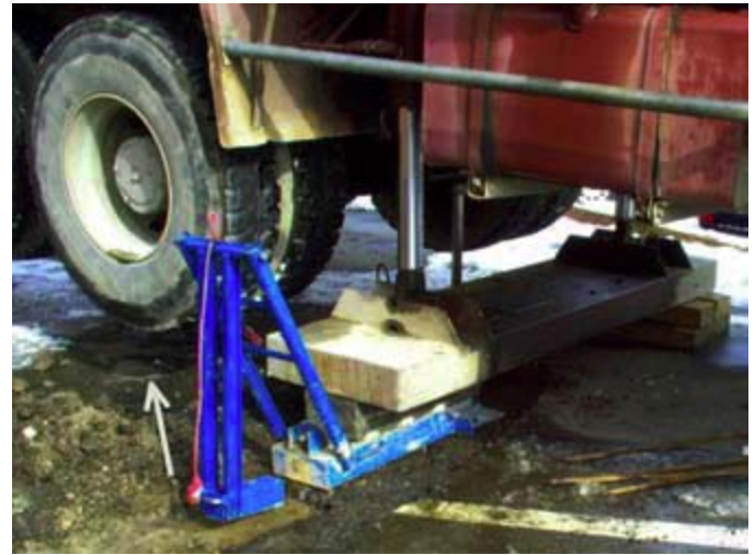
Fig. 3. Shear wave source at the surface.
