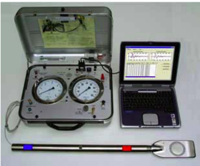
Fig. 2. Seismic dilatometer equipment.
