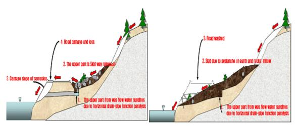
Fig 15. Road breakage by the boulder flow
