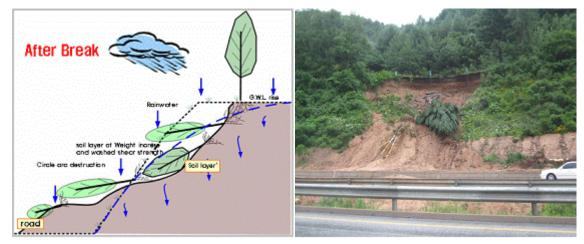
Fig 7. Schematic of arc type failure
