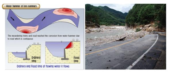
Fig 11. Schematic of water-impacting portion
