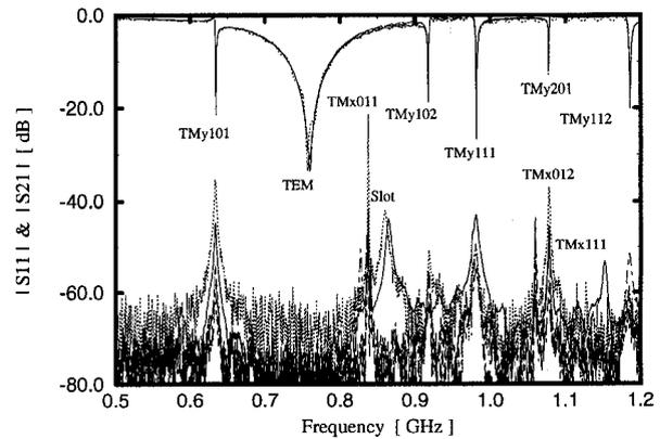
**Figure 6.**  $|S_{11}|$  and  $|S_{21}|$  for different front panels and #5 opened in the center plane CP7 (solid line: FP2; dotted line: FP4M; dashed line: FP5R; long-dashed line: FP6VL; long-short dashed line: FP6HD)
