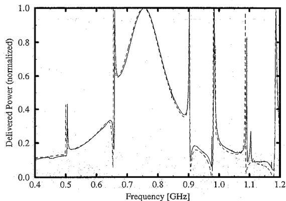
Figure 7. Power delivered to the enclosure calculated from  $|S_{11}|$  measurements (solid line) compared with the FDTD simulation (dashed line); center plane CP4M (with a 30 cm long slot in the middle), the front panel FP2 (with a 40 cm long slot in the bottom), with the width 1 mm for both slots, and feed probe termination of 47.8  $\Omega$ .
