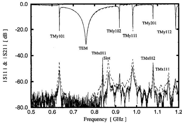
**Figure 4.**  $|S_{11}|$  and  $|S_{21}|$  for the front panel FP2 (30 cm) and different openings in the center plane CP7 (solid line: four squares of  $1\text{ cm}^2$  each in #5; dotted line: one square of  $1\text{ cm}^2$  in #5; dashed line: #5).
