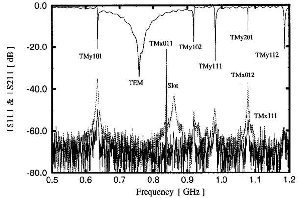
**Figure 5.**  $|S_{11}|$  and  $|S_{21}|$  for the front panel FP4M (30 cm horizontal slot in the middle) and different openings in the center plane CP7 (solid line: one square of  $1\text{ cm}^2$  in #5; dotted line: #5).
