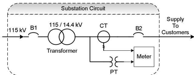
Figure 2. Substation circuit and data acquisition schematic
