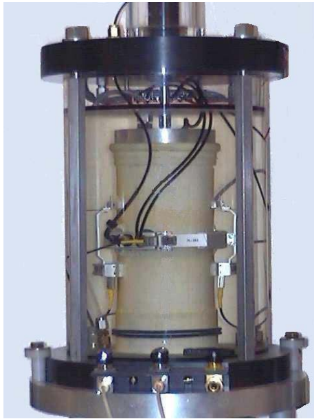
Fig. 3. Triaxial Testing Equipment (Ng and Leung 2007)
