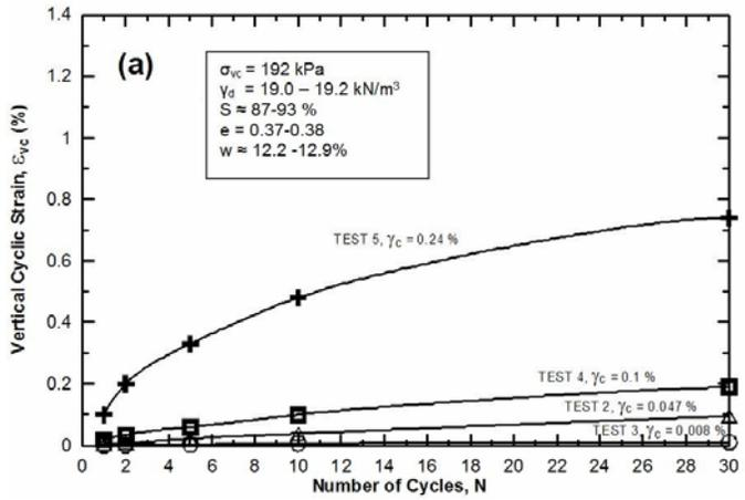
(a) Accumulation of  $\epsilon_{vc}$  with  $N$  for different  $\gamma_c$  applied in different tests.
