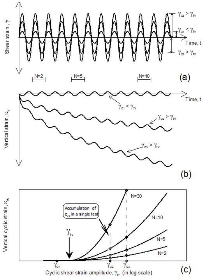
Fig. 2. Sketch of typical results of cyclic simple shear strain-controlled tests: (a) Strain-time histories of three cyclic strain-controlled compression tests; (b) Variation of vertical strain,  $\varepsilon_v$ , with time; (c) Relationship between vertical cyclic strain,  $\varepsilon_{vc}$ , cyclic shear strain amplitude,  $\gamma_c$ , and the number of cycles,  $N$ , obtained from the results of three cyclic strain-controlled compression tests.
