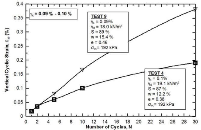
Fig. 8. Effect of dry unit weight,  $\gamma_d$  on  $\epsilon_{vc}$ .
