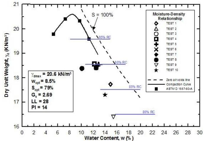
Fig. 6. Dry unit weight,  $\gamma_d$ , versus water content,  $w$ , chart with the modified compaction curve and data points corresponding to the conditions of specimens prior to the application of vertical consolidation stress.
