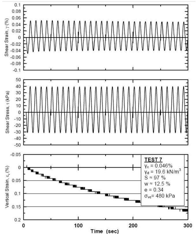
Fig. 4. Typical test results – Test 7
