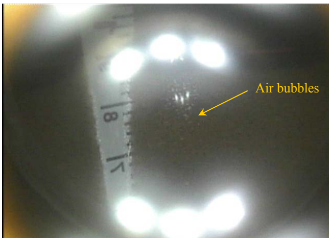
Photo 2. Existence of air bubbles after shaking test
