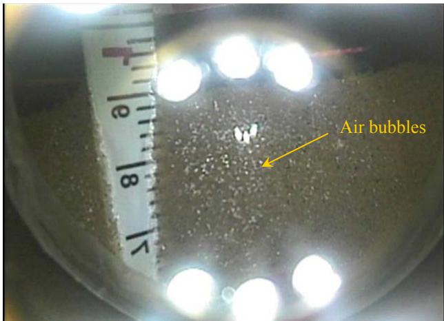
Photo 1. Existence of air bubbles before shaking test
