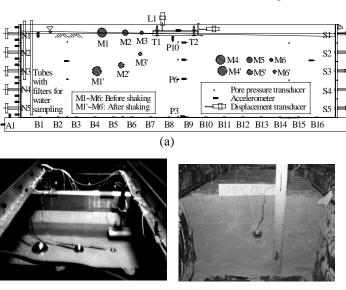
Fig. 8. Geotechnical centrifuge model test: (a) model with instrument layout for in-flight condition; (b) before shaking; (c) soil dissection after shaking. The final positions of the target objects from model dissection after the centrifuge testing are also shown in (a) (M1' ~ M6').
