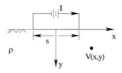
Fig. 1. Infinite half space with current injected from two surface electrodes.
