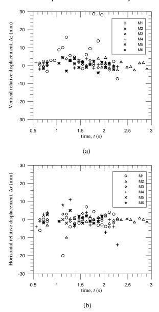
Fig. 10. Calculated relative displacement of M1~M6 (mm) (a) vertical,  $\Delta z$ ; (b) horizontal,  $\Delta x$  vs. time (s).
