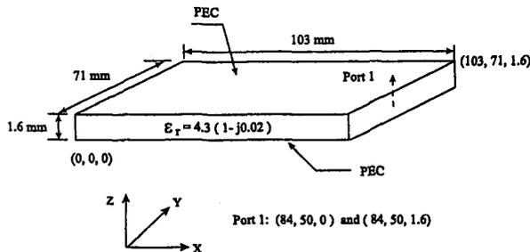
Figure 2. Geometry of a patch antenna
