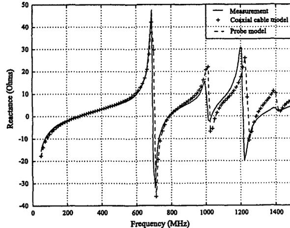
Figure 4. The input reactance of the patch antenna
