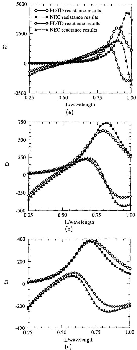
Figure 5: Input impedance comparison between FDTD results and NEC results for a dipole antenna with set source and conductor radii for a) *very thin*,  $a = 0.002\Delta l = \frac{\lambda_0}{21,000}$ , b) *thin*,  $a = 0.2\Delta l = \frac{\lambda_0}{210}$ , c) *thick*,  $a = 0.48\Delta l = \frac{\lambda_0}{87.5}$  wires.
