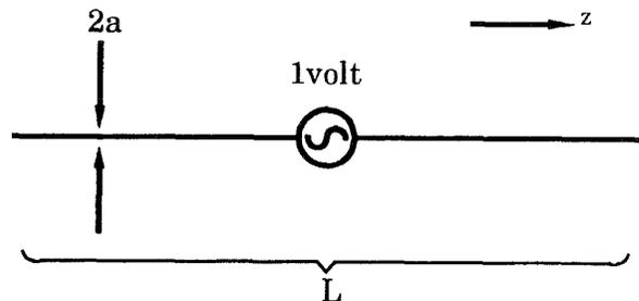
Figure 2: Geometry of the dipole antenna model.
