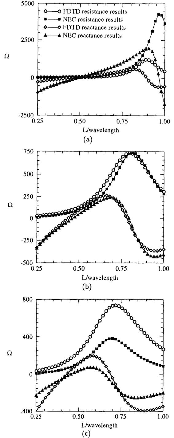
Figure 4: Input impedance comparison between FDTD results and NEC results for a dipole antenna with a set conductor radius, but no defined source radius for a) *very thin*,  $a = 0.002\Delta l = \frac{\lambda_a}{21,000}$ , b) *thin*,  $a = 0.2\Delta l = \frac{\lambda_a}{210}$ , and c) *thick*,  $a = 0.48\Delta l = \frac{\lambda_a}{87.5}$  wires.
