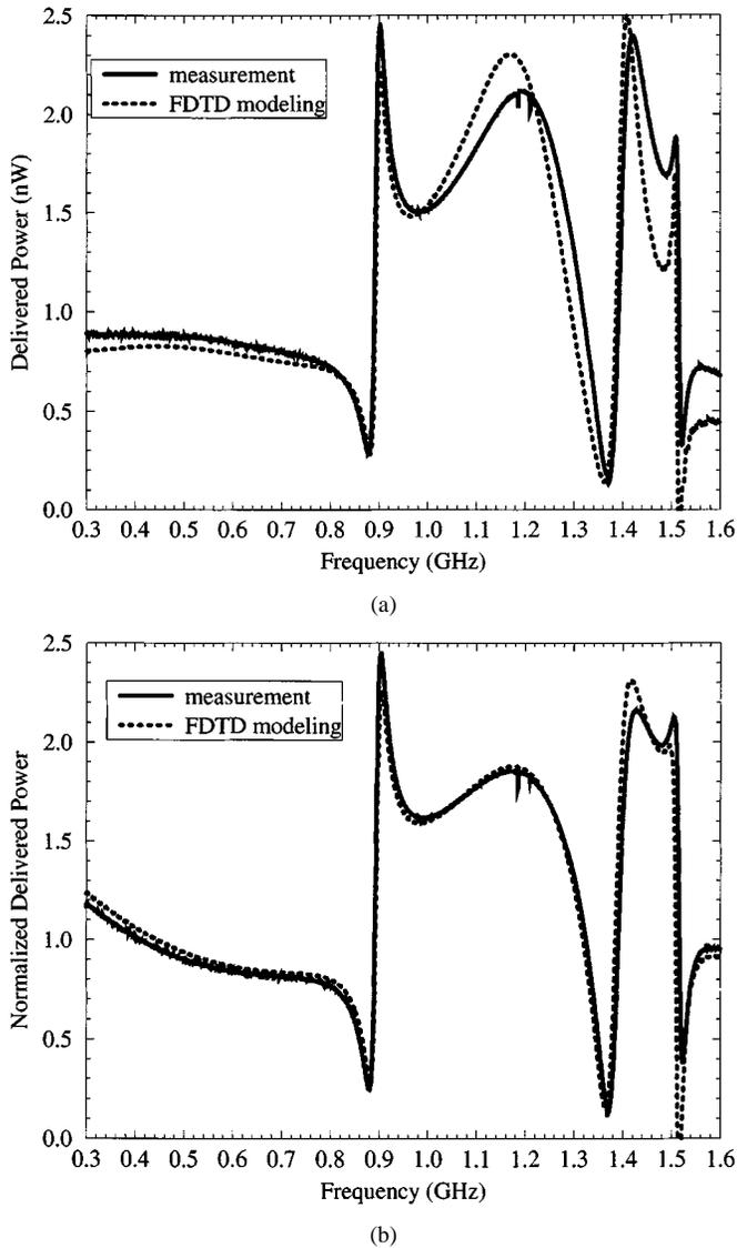
Fig. 9. Comparison between measurements and FDTD modeling for the enclosure configuration without the slot for (a) Ferrite 2 and (b) a 180- $\Omega$  resistor terminating the feed probe.
