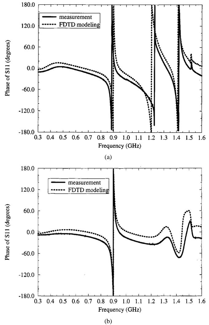
Fig. 10. Comparison of  $\angle S_{11}$  between measurements and FDTD modeling for the enclosure configuration without the slot for (a) Ferrite 1 and a (b) 360- $\Omega$  resistor terminating the feed probe.
