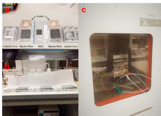
Fig. 1 the pictures of fuel cell stack: a) the disassembled single cell unit; b) the stack covers; c) the three-single-cell stack during the performance test
