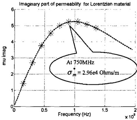
Figure 7. "Points" of  $\sigma_m^*$  taken at the dispersive permeability curve for normal Yee's algorithm.
