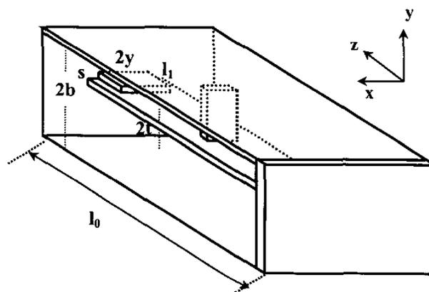
Figure 1. NIST stripline cavity for permittivity and permeability measurements.
