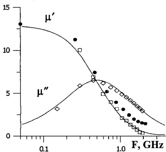
Figure 2. Real and imaginary parts of Ni-Zn ferrite permeability.
