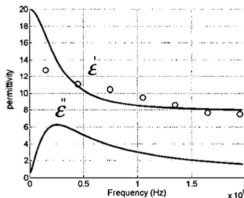
Figure 3. Real and imaginary parts of Ni-Zn ferrite permittivity.
