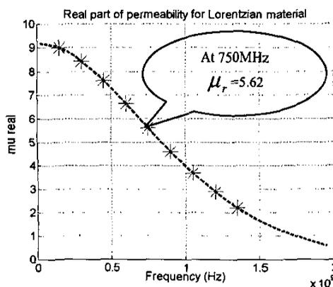
Figure 6. “Points” of  $\mu_r$  taken at the dispersive permeability curve for normal Yee’s algorithm.
