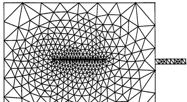
**Figure 6: Example of the board mesh for the FEM/MOM hybrid model.**
