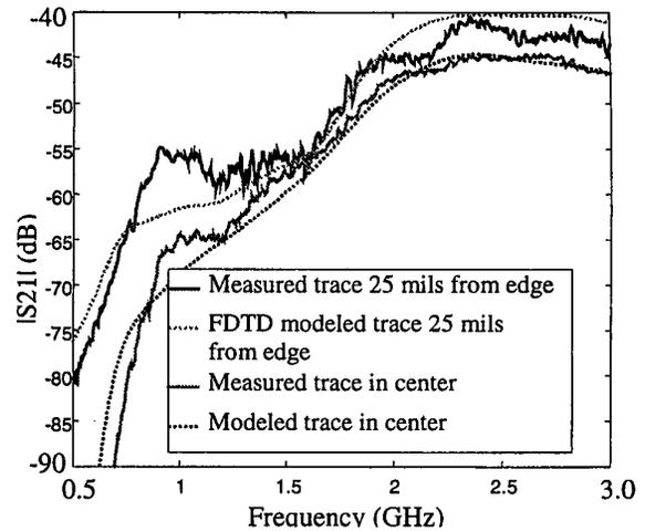
**Figure 5: Comparison of FDTD and measured results for a centered trace and a trace near the edge with  $d = 25\text{ mils}$ .**
