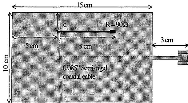
Figure 1: Geometry of PCB layout.
