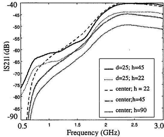
Figure 8: Comparison of the near-electric field radiation for different trace heights above the reference plane for a centered trace, and trace 25 mils from edge.
