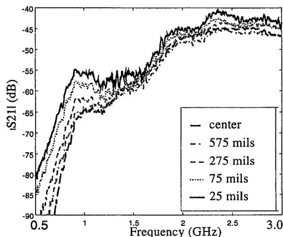
**Figure 4:  $|S_{21}|$  measurements using a 3 cm monopole probe.**
