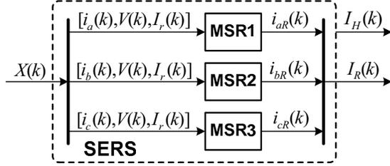
Fig. 5. Structure of the sensor evaluation and restoration scheme (SERS):  $X = [I, V, I_r]$ ,  $I = [i_a, i_b, i_c]$ ,  $V = [v_{ca}, v_{cb}, v_{cc}]$ , and  $I_r = [i_{ra}, i_{rb}, i_{rc}]$ .
