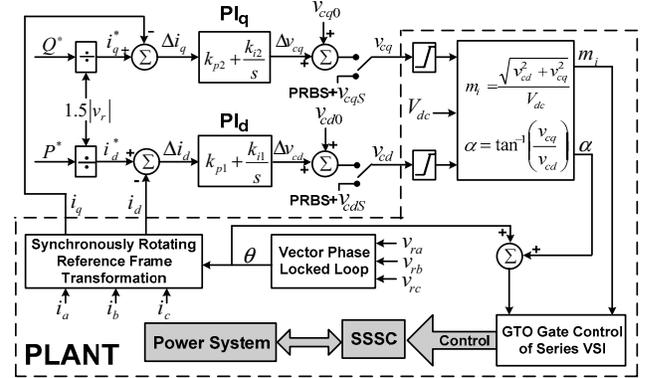
Fig. 3.  $P$ - $Q$  decoupled control scheme for SSSC
