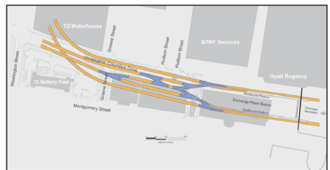
Fig. 7 Exchange Place Cross-Overs
