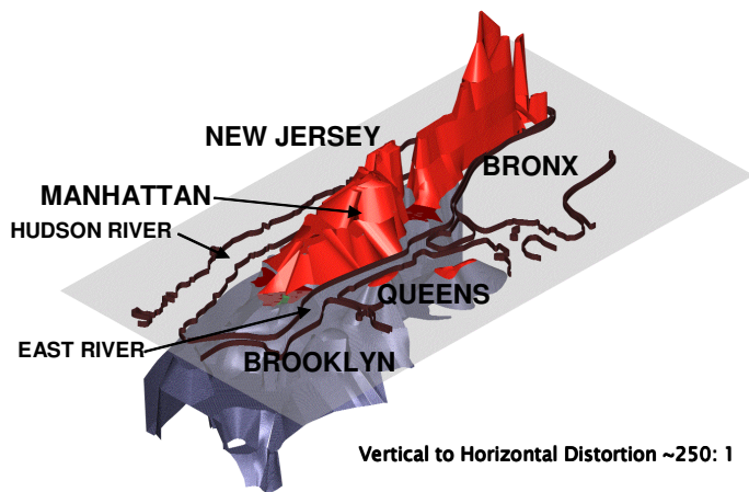
Fig. 3. Manhattan bedrock subsurface (developed by Mueser Rutledge Consulting Engineers, 2000).
