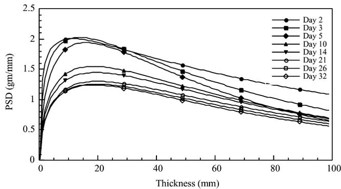
Fig. 10. Pore solution distribution in the cube for cycle 2.
