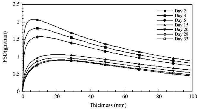
Fig. 6. Pore solution distribution in the cube for cycle 1.
