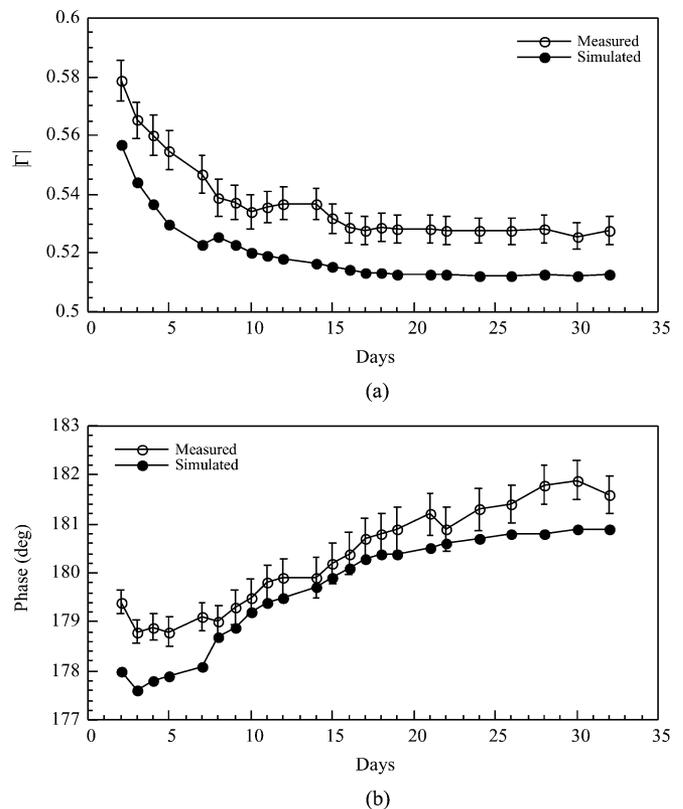
Fig. 11. Comparison of the measured and simulated reflection coefficient of the cube at 3 GHz and for cycle 2 (a) magnitude and (b) phase.
