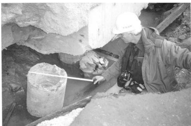
Fig.3. Shearing of a pile by ground displacements in 1995 Kobe earthquake (Finn and Fujita 2002).
