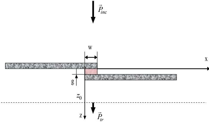
**Figure 4.** Geometry of the problem:  $w= 50$  mm and  $g = 3$  mm.
