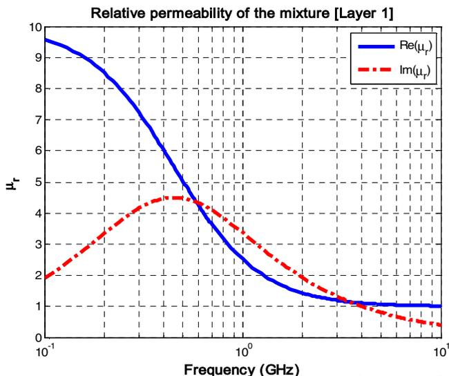
**Figure 2.** Permeability of the mixture as a function of frequency. The mixture contains 30% of Ni-Zn ferrite with magnetic parameters:  $\mu_{sf} = 45$ ,  $f_{rf} = \frac{1}{2\pi\tau_{fm}} = 450$  MHz.
