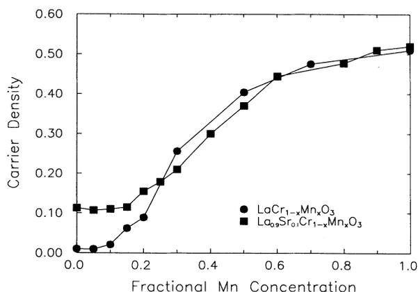
FIG. 3. Carrier density vs Mn content at 1300 K for the series  $\text{La}(\text{Cr},\text{Mn})\text{O}_3$  and  $\text{La}_{0.9}\text{Sr}_{0.1}(\text{Cr},\text{Mn})\text{O}_3$ , as ascertained by the application of Heikes's formula to the Seebeck coefficient data of Figs. 2 and 7.
