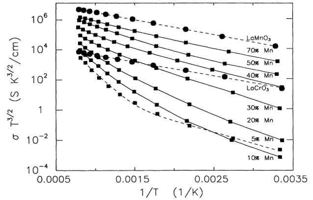
FIG. 1. Logarithmic plot of  $\sigma T^{3/2}$  as a function of inverse temperature for the series La(Cr,Mn)O<sub>3</sub>. Circles represent end members and squares represent mixed samples. Dashed lines are theoretical fits to the data.
