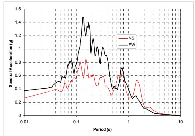
Fig. 2. Acceleration response spectra for horizontal components of ground motion recorded at the Manzanillo Power Plant (Damping = 5%).
