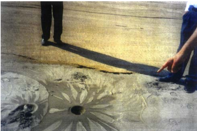
Fig. 5. Wet hole on February 11, 2001 from which water and silt had oozed out
