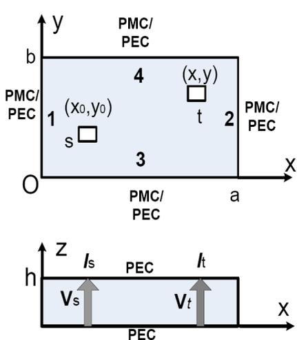
Figure 1. Various possible cavity boundaries for RFI analysis.
