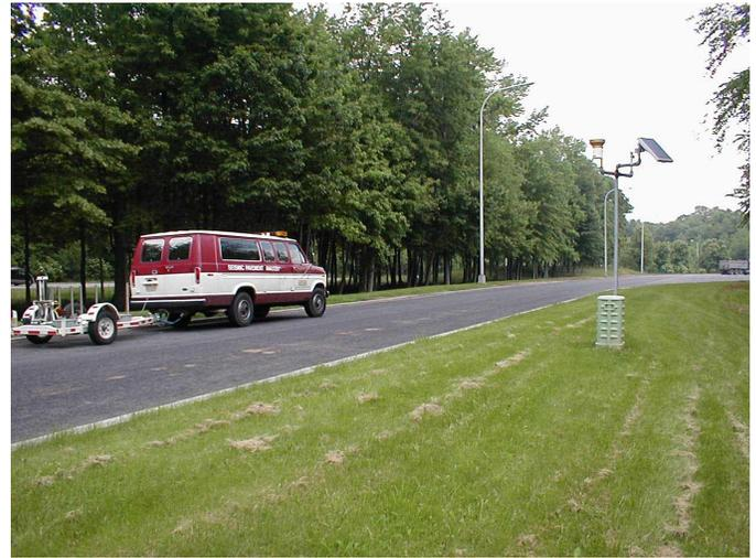
Fig. 3. SPA testing on test section 4. Instrumentation cabinet and climate measurement pole are visible at the right part of the picture.
