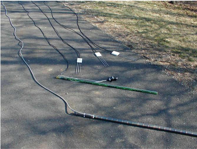
Fig. 2. TDR (top), temperature (middle), and resistivity (bottom) probes to be installed in test section 3.
