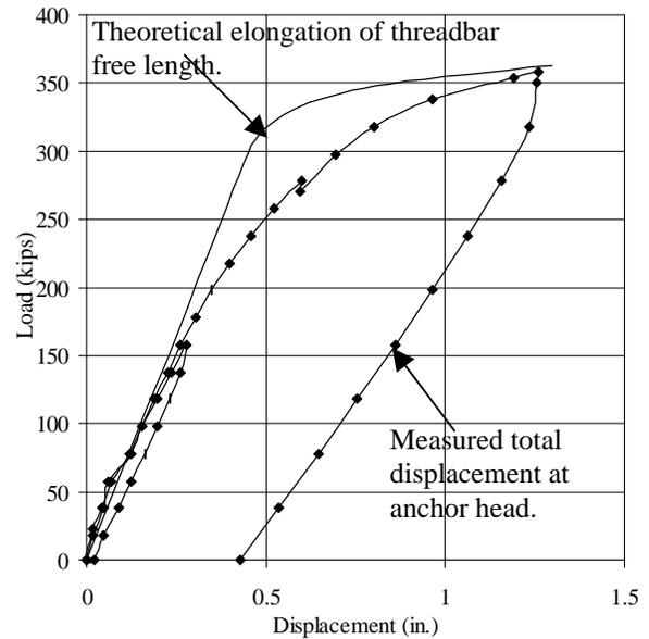
Fig. 2. Load Vs Displacement of Cement-Grout Anchor B-8.
