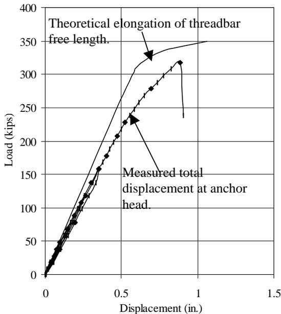
Fig. 3. Load Vs Displacement of Cement-Grout Anchor B-6.
