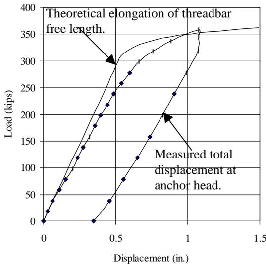
Fig.1. Load Vs Displacement of Resin Anchor B-1.
