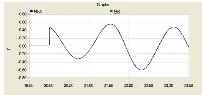
Figure 21. Actual speed deviation of generator G2 and the estimated output of the ID\_Gen\_Speed\_Net2 when PRBS signals are applied to G2's excitation and turbine at 20s with fixed weights of ID\_Gen\_Speed\_Net1.
