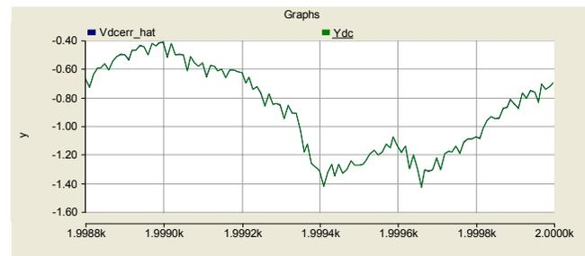
Figure 23. Actual UPFC dc capacitor voltage deviation and the estimated output of the ID\_DC\_Voltage\_Net (with fixed weights) when PRBS signals are applied to shunt bus voltage reference  $V_{AREF}$  and dc capacitor voltage reference  $V_{dcREF}$  and training have been terminated at 1900s.
