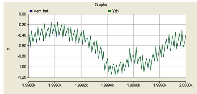
Figure 22. Actual UPFC shunt bus voltage deviation and the estimated output of the ID\_Bus\_Voltage\_Net (with fixed weights) when PRBS signals are applied to shunt bus voltage reference  $V_{AREF}$  and dc capacitor voltage reference  $V_{dcREF}$  and training have been terminated at 1900s.
