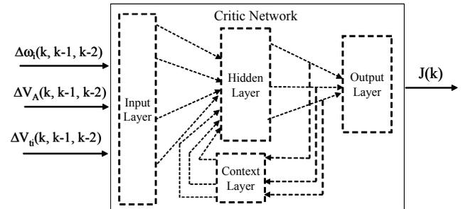
Figure 8. A recurrent neural network implementation for the critic network in Fig. 7 with 34 inputs at time instances  $k+1$ ,  $k$  and  $k-1$  in the input layer, 25 inputs in the context layer from the outputs of the 25 sigmoidal neurons in the hidden layer.
