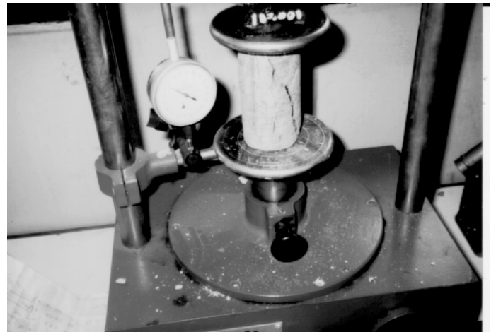
Fig. 9. Unconfined compression test of jet grouted sample.
