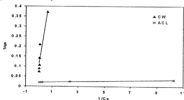
**Fig. 9: Langmuir Isotherm for Removal of Pyridine**
