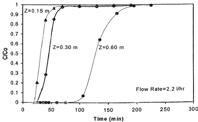
**Fig. 11: Breakthrough Curves for Removal of Pyridine by Bagasse Fly Ash**
