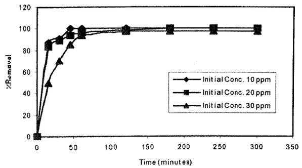
**Fig. 6: Effect of Contact Time and initial concentration (Ci) on Removal of 3-Picoline using carbon waste as adsorbent**
