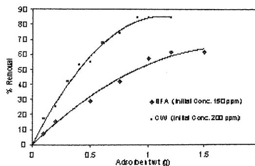
Fig. 4: Effect of Adsorbent Dose on Removal of Pyridine
