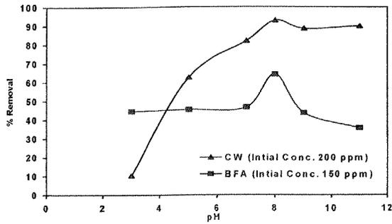
**Fig. 5: Effect of pH on Removal of Pyridine**
