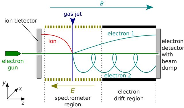
FIG. 2. Schematic drawing of the employed reaction microscope.
