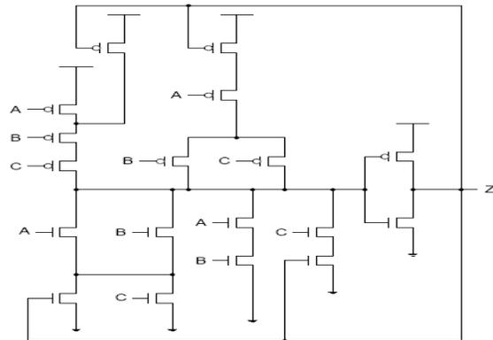
Fig. 2: Static CMOS implementation of TH23 gate
