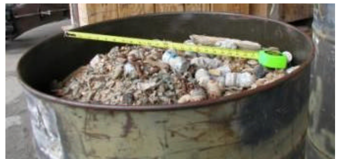
Fig. 2 – Oversized Projectile Fragments Removed From ATF Soil Impact Berms
