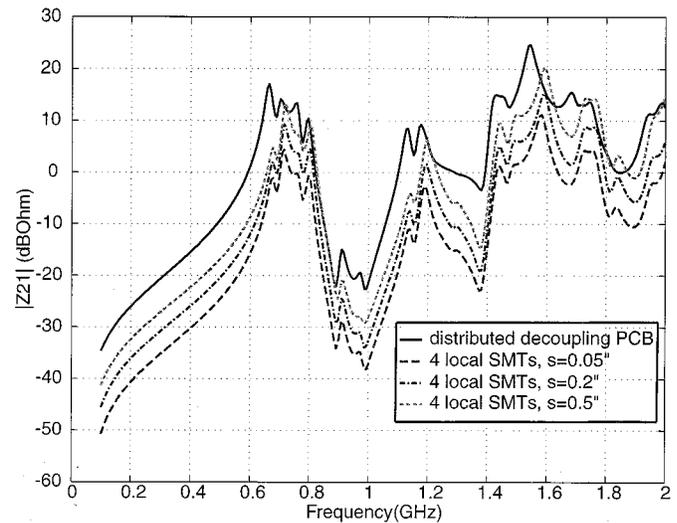
Fig. 9. Local SMT decoupling effect versus spacing.
