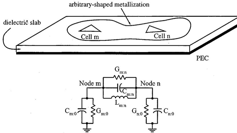
Fig. 2. The equivalent circuit model between any arbitrary pair of two nodes  $m$  and  $n$ .
