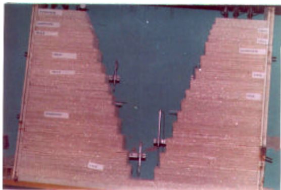
Fig 2. Excavation down to 14 th bench (141.0 cm depth).
