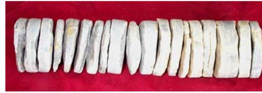
Fig. 1. Rock disk produced in drilling
