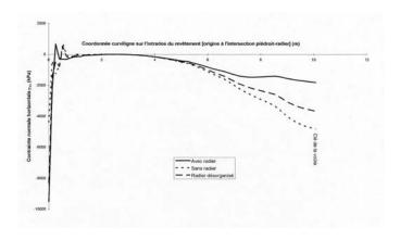
Fig. 8a. Variation of the horizontal normal stress  $\sigma_{xx}$  along the tunnel intrados
