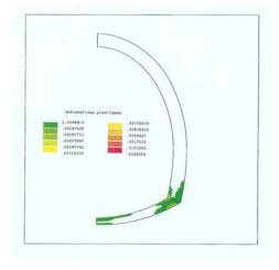
Fig. 9c. Isovalues of total plastic strain for the analysis with disorganized invert
