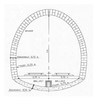
Fig. 1. Typical tunnel section
