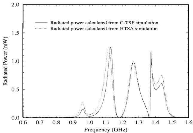
Fig. 13. Comparison of HTSA and C-TSF FDTD simulations for the power radiated through the slot.
