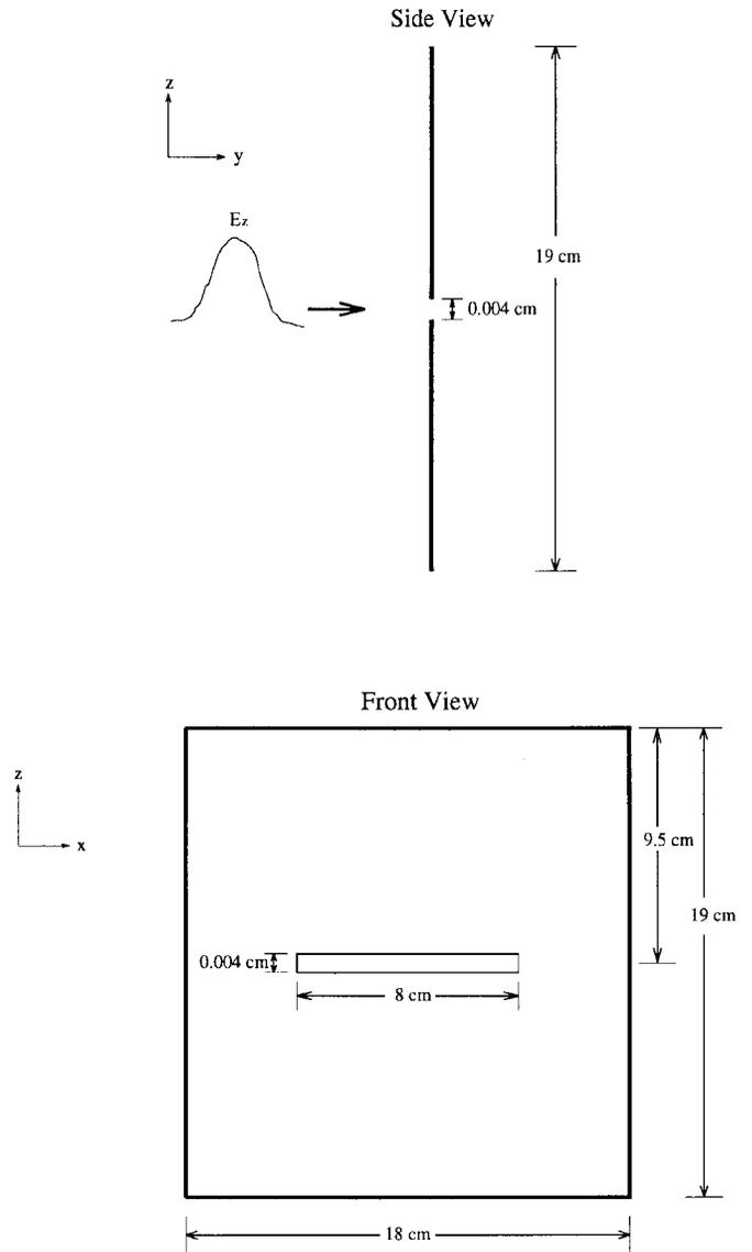
Fig. 7. The geometry of the 3-D finite plate.
