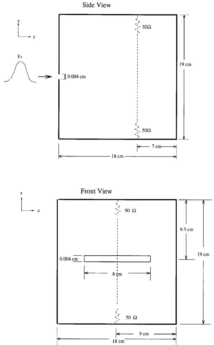
Fig. 9. The geometry of the loaded cavity.
