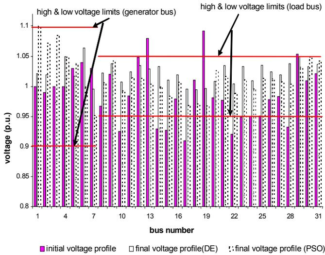
Fig. 1: Voltage profile correction for DE and PSO
