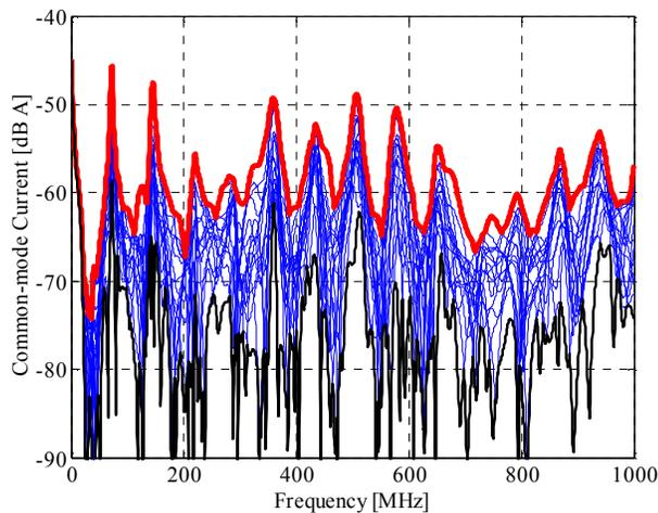
Fig. 6. Amplitude of the sixteen simulated CM currents at point P1.
