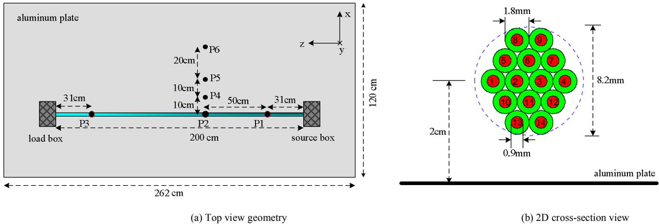
Fig. 4. Schematic of the measurement setup, (a) top view geometry, (b) 2D cross-section view. The CM current was simulated and measured at point P1, P2 and P3, and the electric field was simulated and measured at point P4, P5 and P6.
