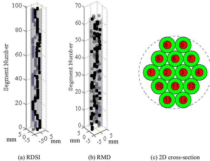
Fig. 2. 3D visualization of two wires along the bundle that are constructed with the RDSI and RMD algorithm: (a) RDSI, (b) RMD, and (c) 2D cross-section. Note that for both algorithms, the normalized STDs are 0.5, and the bundle lengths are both two meters long.
