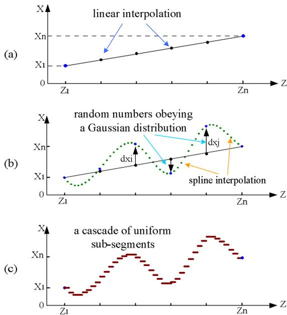
Fig. 1. Schematic representation of wire modeling using the Random Displacement Spline Interpolation (RDSI) algorithm.
