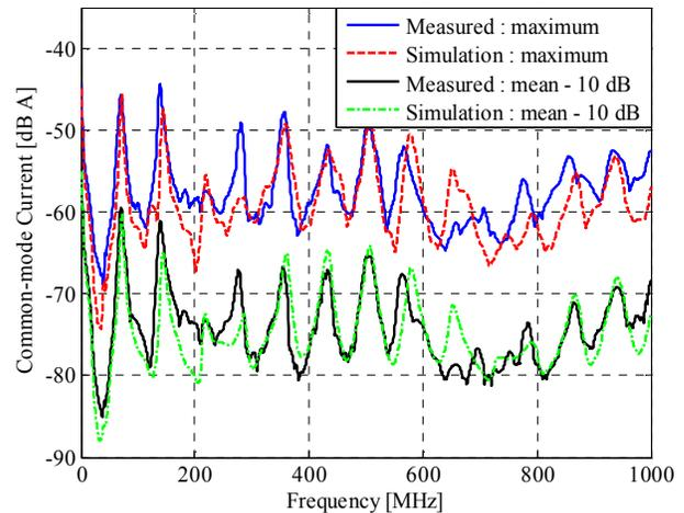
Fig. 7. Comparison of the measured and simulated maximum and average CM current at point P1. Note that both the simulated and measured average CM currents are shifted 10 dB down from the original values for ease of comparison.
