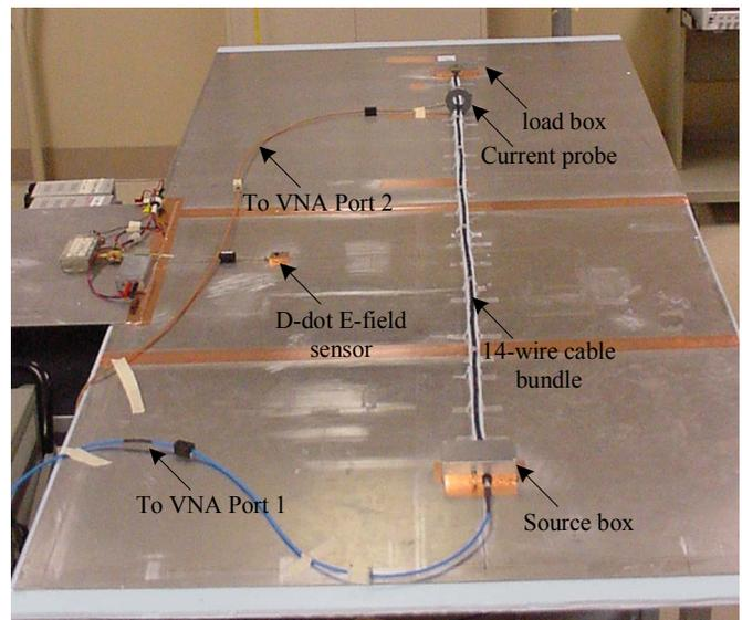
Fig. 3. Photograph of the measurement setup for a fourteen-wire, two-meter long cable harness over a large aluminum plate.
