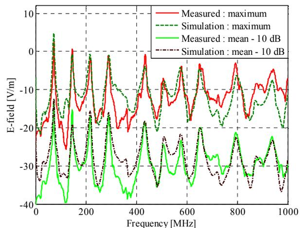
Fig. 8. Comparison of the measured and simulated maximum and average electric field at point P4. Note that both the simulated and measured average E-field data are shifted 10 dB down from the original values for ease of comparison.
