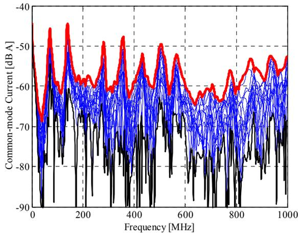
Fig. 5. Amplitude of the sixteen measured CM currents at point P1.
