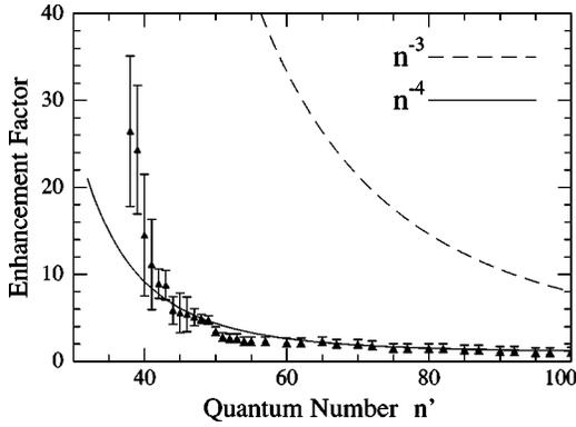
FIG. 3. The enhancement factor in the stabilization of the doubly excited states versus the final Rydberg state principle quantum number ( $n'$ ) due to the application of the second short laser pulse is shown. The dashed curve represents our theoretical calculation for the case when no static electric field was present in the interaction region. The solid curve represents the calculation when a small static field ( $\sim 5$  V/cm) was present in the interaction region.
