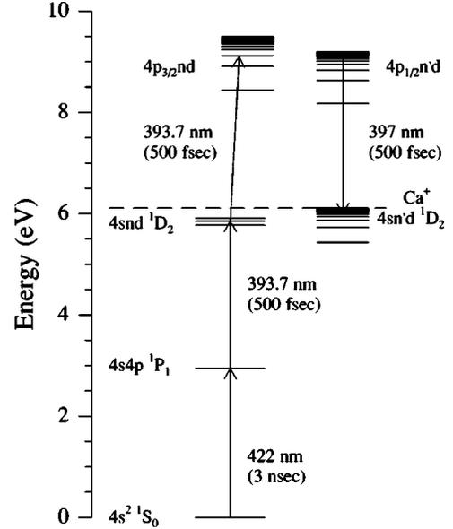
FIG. 1. Excitation diagram for calcium used in the experiment. The first nanosecond dye laser excites the  $4s^2 1S_0$  ground state to the  $4s4p 1P_1$ . About 4 nsec later, a 500-fsec laser pulse promotes the atoms via a two-photon resonant transition to a pure  $4p_{3/2}nd$  doubly excited state, where  $n=20, 21,$  and  $22$ . A second 500-fsec laser short pulse was then used to drive the transition from the  $4p_{1/2}n'd$  states to the  $4sn'd$  states.
