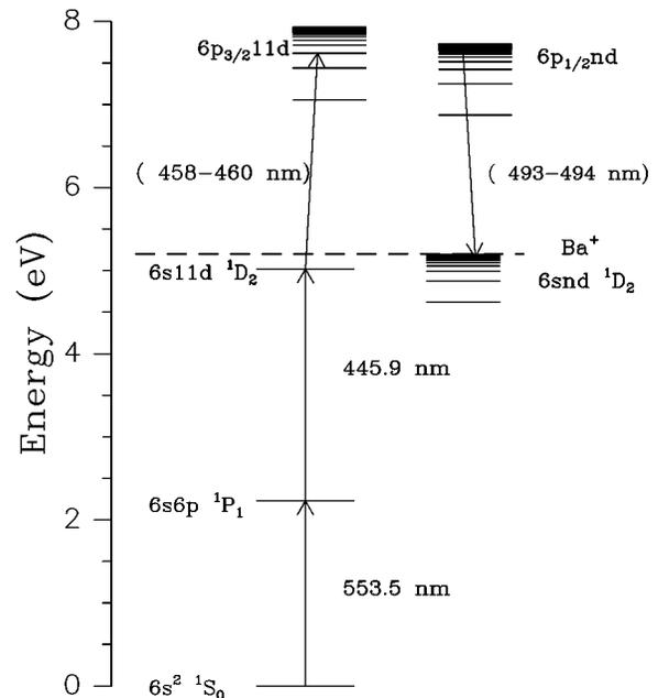
FIG. 1. Energy levels of barium involved in the experiment are shown along with the relevant laser transitions. Two photons were used to excite the  $6s11d\ ^1D_2$  state. A third laser then excited a doubly excited state in the energy range of  $6p_{1/2}nd$  Rydberg series. A fourth laser was used to drive the transition from the  $6p_{1/2}nd$  states to the  $6snd$  states.
