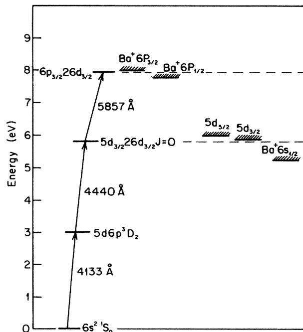
FIG. 1. Barium energy-level diagram showing the excitation scheme to populate the  $5d_{3/2}26d_{3/2}$ ,  $J=0$  state. The third laser monitors the metastable population by further exciting the atoms to the autoionizing  $6p_{3/2}26d_{3/2}$ ,  $J=1$  state.
